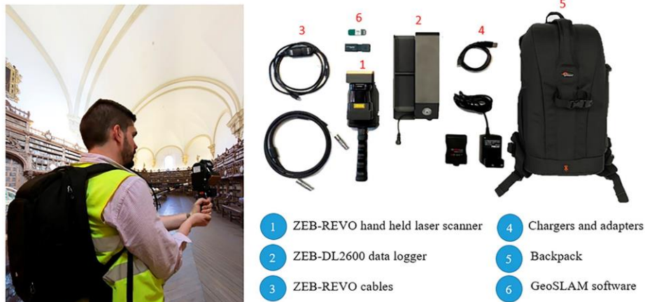
Fig. 2. WMMS used: a) user working with the wearable laser scan (Zeb-Revo). b) Zeb-Revo equipment.
