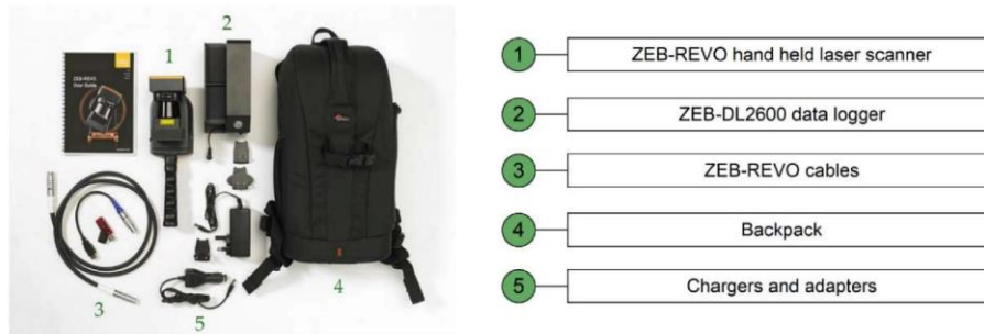
Figure 1. Main components of the wearable mobile laser systems (WMLS) used for data acquisition.
