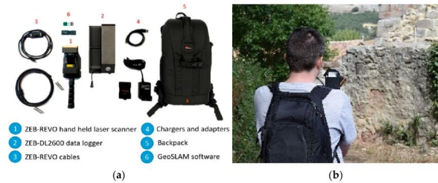
Figure 5. Wearable mobile mapping system used: (a) main components and (b) photo taken during the data acquisition.
