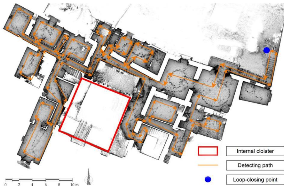
Figure 3. Example of a survey design with the WMLS. The compensation of the accumulated error is possible thanks to the closure of the path following different track and acquiring the internal cloister area from different points of the route.
