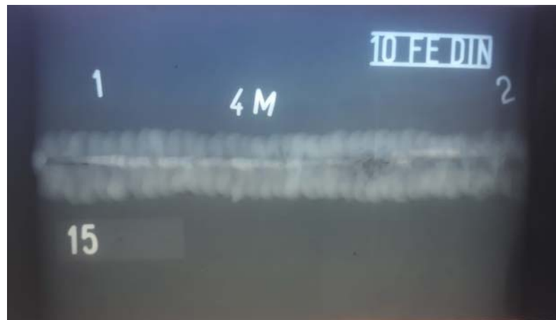
Figure 4. Real X-ray radiography of a metallic weld with defects (lack of fusion and vermicular pores).
