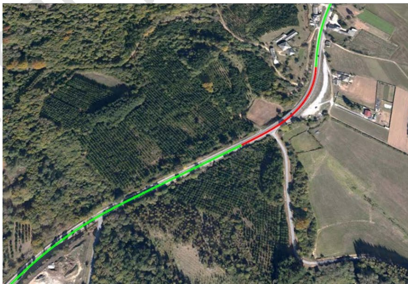
523 Fig. 7. Risk mapping for the different geometric elements of the horizontal alignment. Case study 1 LU- 524 722 Stretch 1. Red line: High risk. Orange line: Medium risk. Green line: Low risk.
