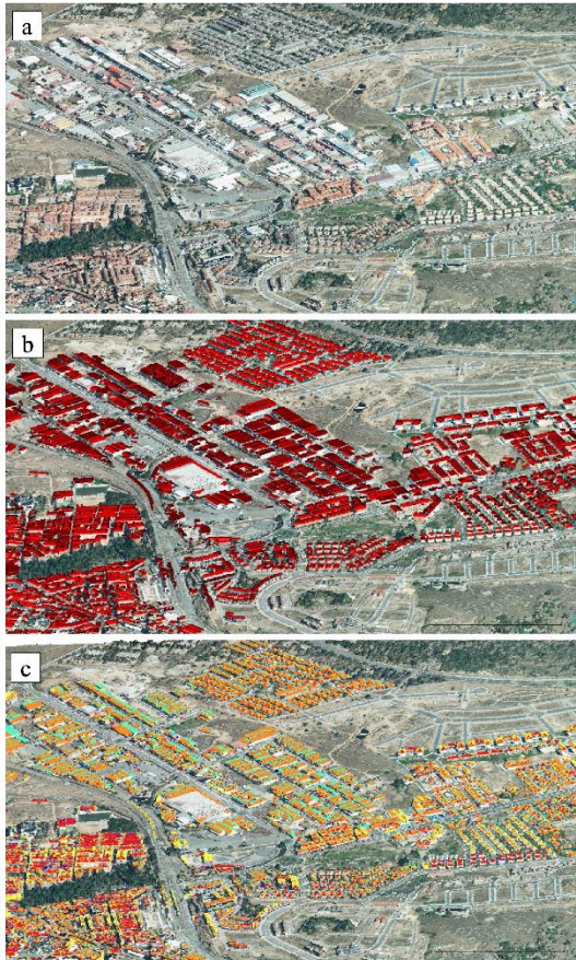
Fig. 8. Perspective view of part of the city of Ávila. (a) Raw LiDAR point cloud with true RGB values. (b) Incorporation of the roof layer in red. (c) Roof layer colorized according to the azimuth-orientation of roofs and with information about their tilt angles. (For interpretation of the references to colour in this figure legend, the reader is referred to the web version of this article.)
