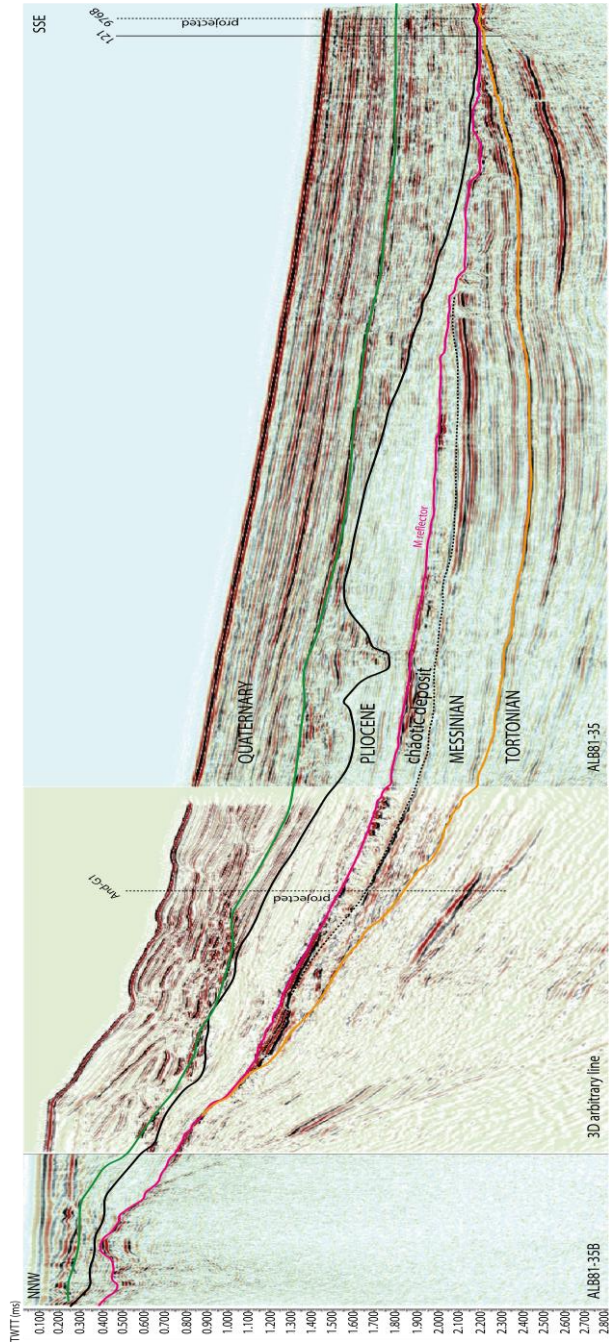
Figure 3: Composite seismic profile (ALB81-35B, 3D arbitrary line and line ALB81-35) showing with a full line, the DSDP Site 121 and with a dashed one the projection of ODP 976 Site and And-G1 industrial well. The colored lines show the top of different geological stages: in yellow: top Tortonian; in black dashed: base of the chaotic deposit; in magenta: top Messinian and M reflector; in green: top Pliocene.
