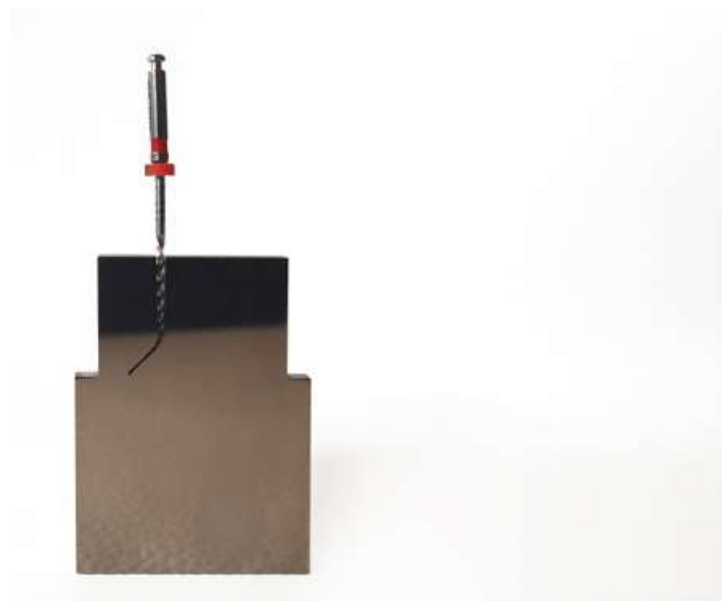
Figure 2. Artificial root canal manufactured from stainless steel with EDM molybdenum wire-cut technology in close contact with a NiTi alloy endodontic rotary file.
