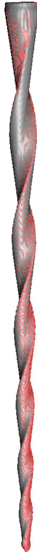
Figure 2. The procedure for alignment between the preoperative (red) and postoperative (grey) digital files and identification of the localization of the CM-wire NiTi alloy endodontic reciprocating files.
