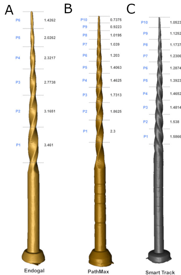
Figure 5. (A) STL digital files of EDG NiTi alloy endodontic rotary file, (B) PMP heat-treated NiTi alloy endodontic rotary file, and (C) ST heat-treated NiTi alloy endodontic reciprocating file.
