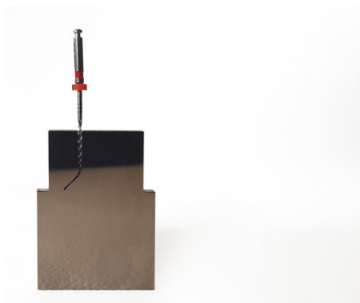
Figure 2. Artificial root canal manufactured from stainless steel with EDM molybdenum wire-cut technology in close contact with a NiTi alloy endodontic rotary file.
