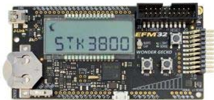
Figura 7. Vista superior de la evaluation board EFM32WG-STK3800
