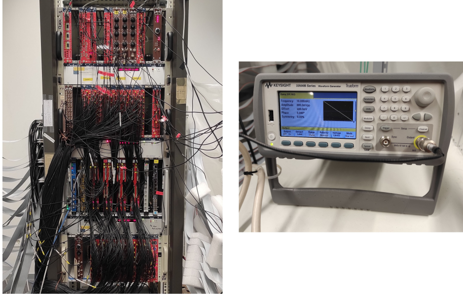
Figure 15: Photographs of the experimental electronic setup. Left: NIM and VME racks where the electronic modules are placed and the cables that establish the connections between them. Right: Signal generator used to create the ramp.
