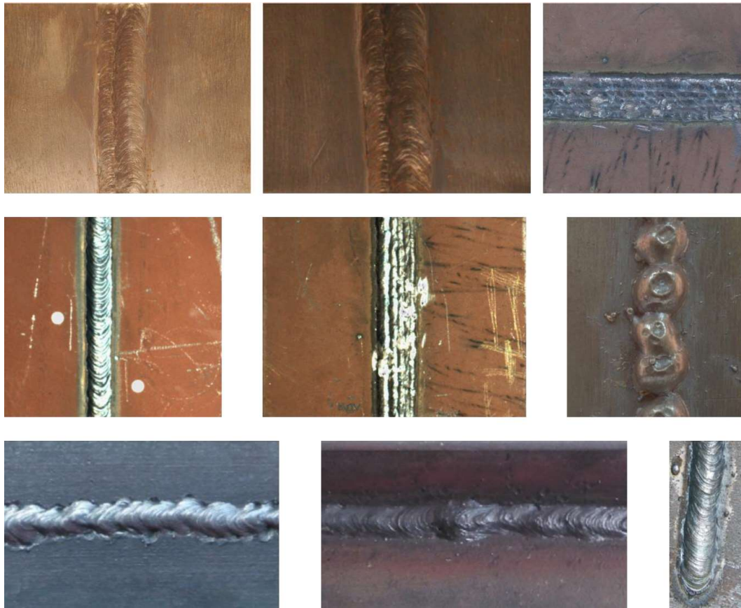
Figure 3. Different types of metallic welds acquired in real scenarios and in the laboratory.
