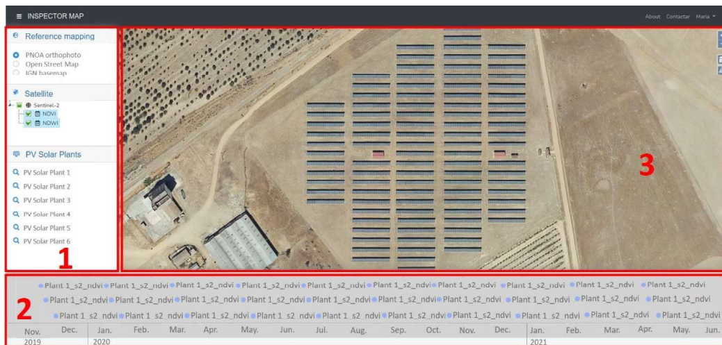
Figure 2. Graphic interface of the SDI INSPECTORMAP developed for the monitoring of photovoltaic plants.
