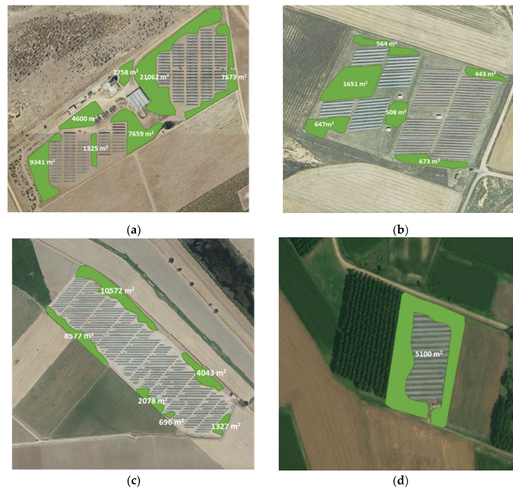
Figure 10. Areas detected and quantified by the INSPECTORMAP alert system for the dates that reveal greater vegetative vigor: (a) plant 1, (b) plant 3, (c) plant 4, and (d) plant 6.
