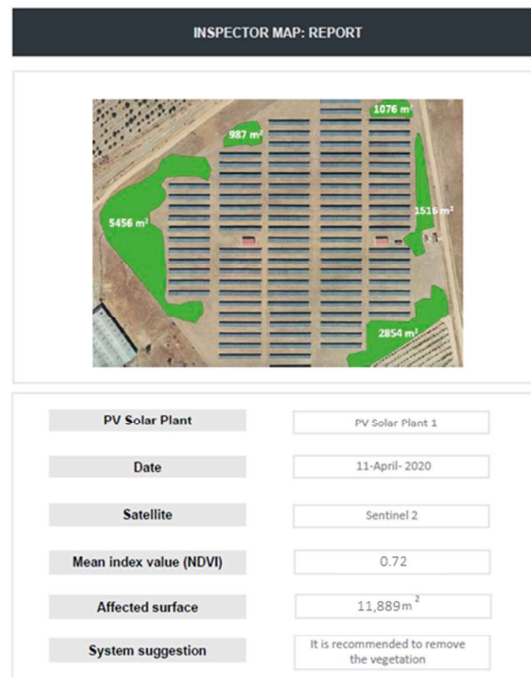
Figure 7. Standard report generated by the SDI INSPECTORMAP when the alert system is activated.
