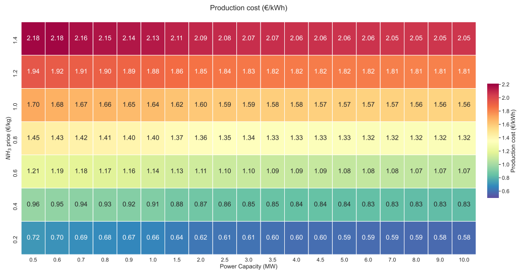
Figure 6: Cost of electricity via the electrochemical conversion of ammonia for different ammonia prices and production capacities
