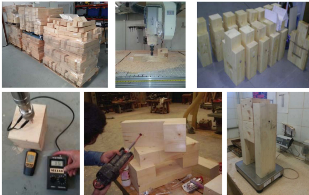
Figure 2. Reception, manufacture, test samples, moisture measurement and conditioning the hole for dowel insertion and weight measurement.
