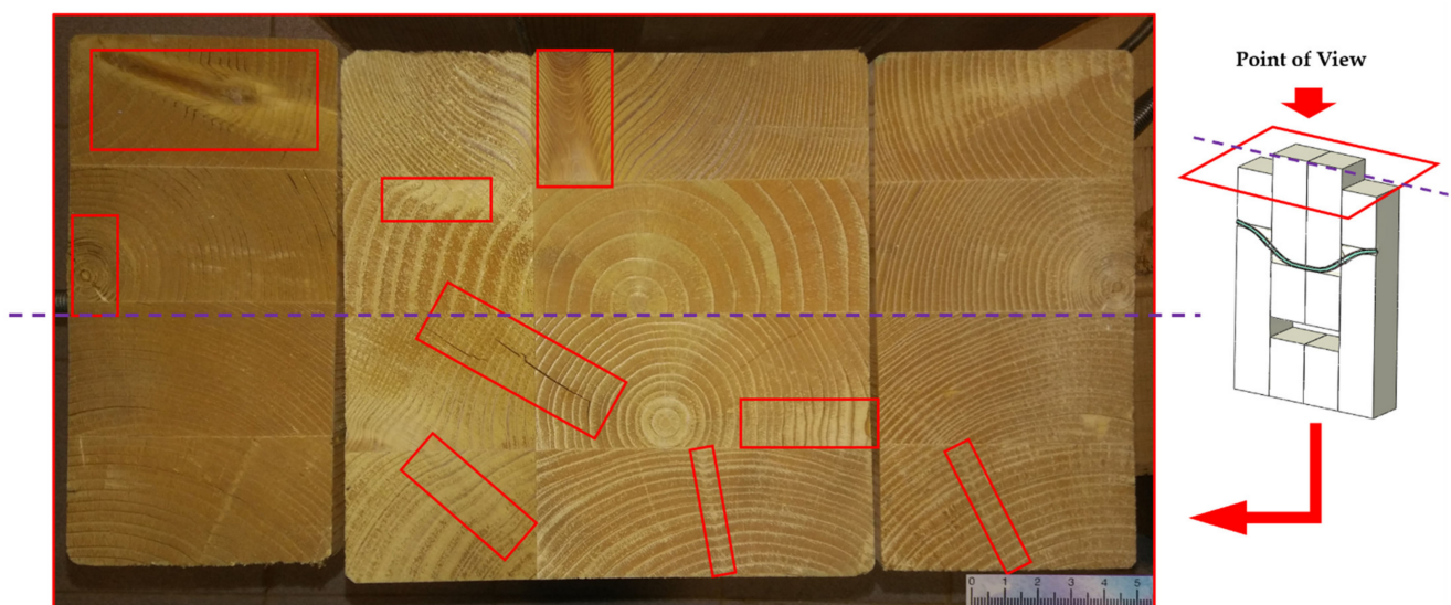
Figure 3. Configuration of timber (unpolished, top view), showing some heterogeneities (marked by red squares) and its plane of symmetry.
