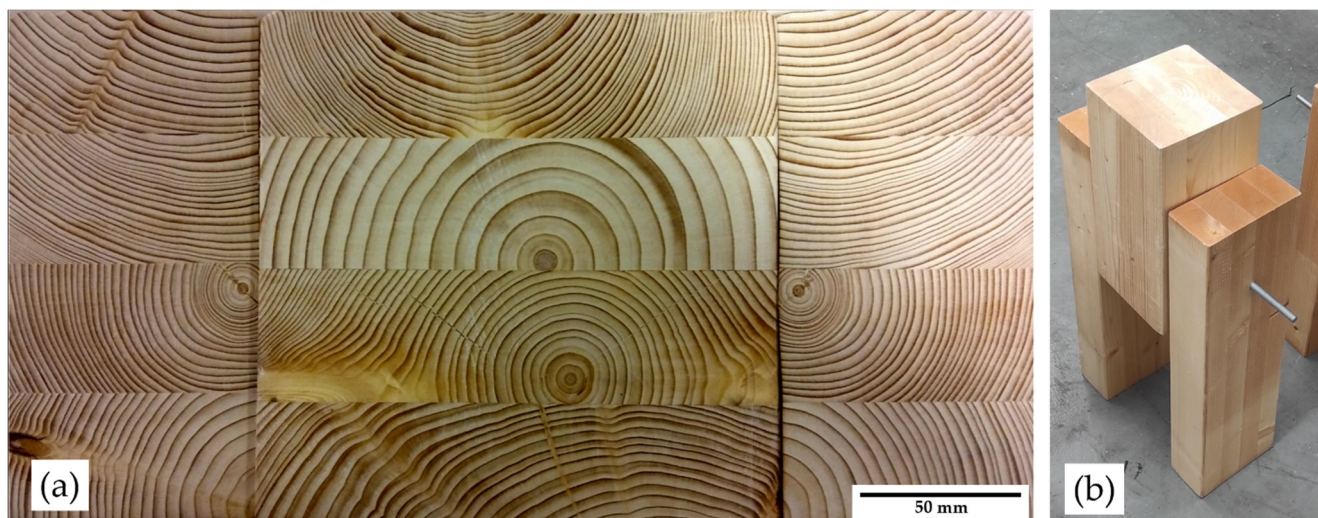
Figure 3. Configuration of the timber (GL24h) used for the tests: (a) detail of the polished sample, upper part of the test specimen, and (b) specimen for the test.
