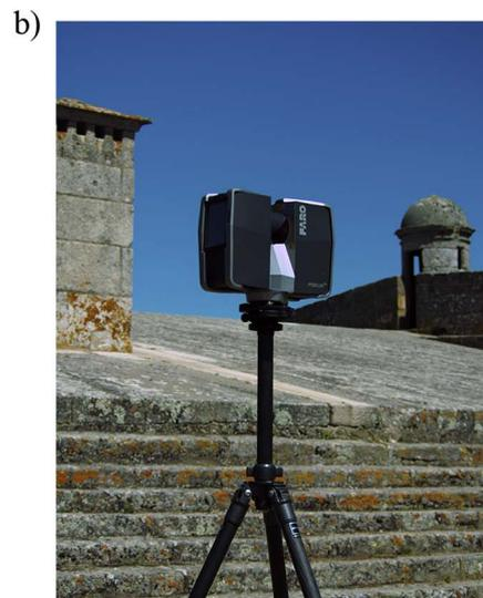
**Fig. 1.** TLS system during the data acquisition: (a) inside the barrel vault and (b) on the roof.
