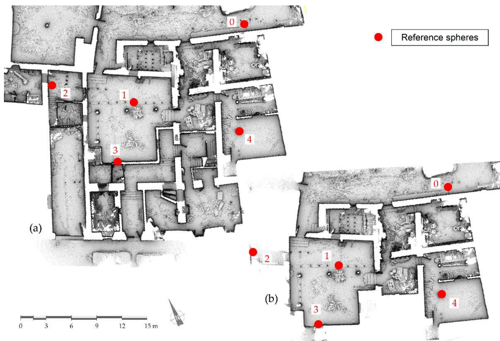
Figure 11. Reference sphere distribution on the ground floor for the path 3 (a) and path 4 (b).
