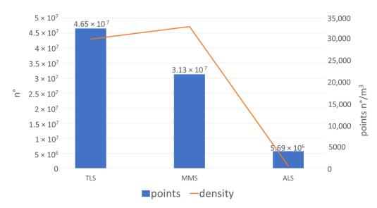
**Figure 12.** Number of cloud points for each original dataset acquired and volume density in 1 m $^3$ . All the data are extracted by an area of 3000 m $^2$ .
