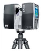
**Figure 6.** Faro Focus 3D X130 Terrestrial Laser Scanner device used for the detailed digitalization of the building and its environment. On the left, the laser scanner is shown during data collection and on the right the equipment in detail.
