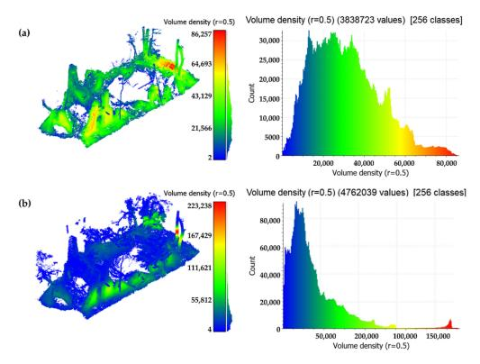
**Figure 13.** Point cloud density expressed in pts/m<sup>3</sup> of TLS data and relative histogram (**a**) with respect to Kaarta Stencil WMMS data (**b**).
