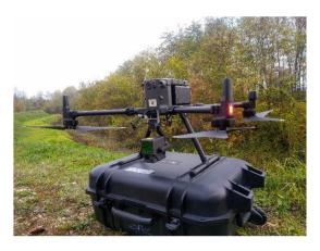
Figure 8. DJI Matrice 300 RTK with DJI Zenmuse L1 ALS.
