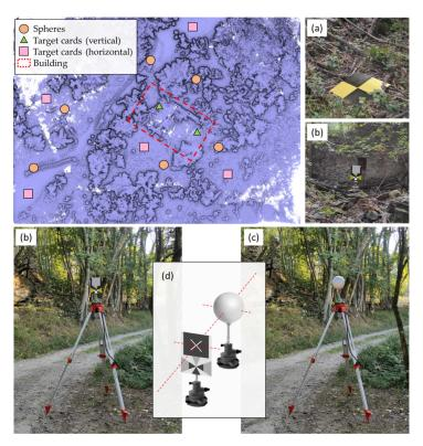
**Figure 9.** Network of registration spheres and target cards (horizontally and vertically), plant view. (a) Horizontal target cards; (b) vertical target cards; (c) spheres; (d) image of the calibration system.
