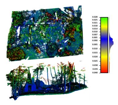
**Figure 14.** Discrepancies obtained from the comparison of the TLS and MMS point clouds. It is observed that most of the MMS point clouds show a blue color, indicating that the discrepancies between the MMSS and the TLS are under or near 1 cm. Yellow, red, and blue areas indicate vegetation zones (with minimal wind, they can move and generate discrepancies between point clouds).
