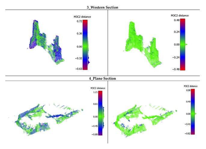
**Figure 18.** *M3C2* analysis of the building along different sections with direct geo-referencing and after ICP. Faro Focus 3D X130 TLS is used as reference and DJI Zenmuse L2 as compared dataset.
