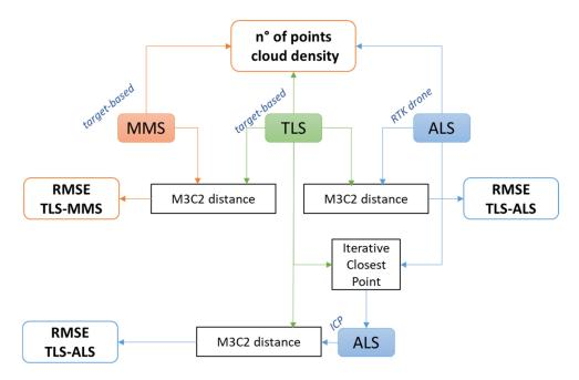
**Figure 4.** Validation analysis workflow to compare FARO Focus 3D X130 TLS, Kaarta Stencil 2–16 MMS, and DJI Zenmuse L1 ALS.
