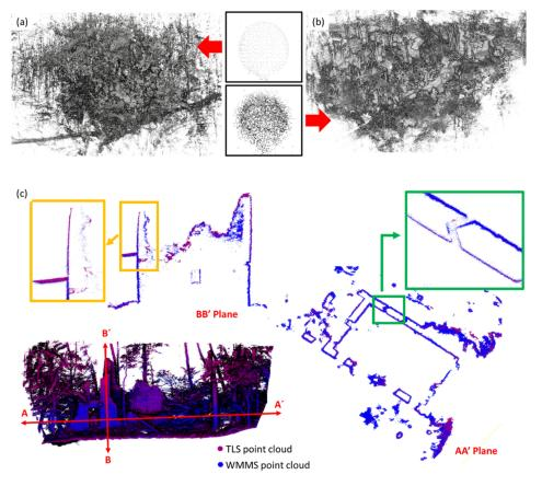
**Figure 15.** (a) TLS point cloud; (b) MMS point cloud; (c) comparison between the TLS and the MMSS point clouds—the TLS point cloud is in purple and the MMS point cloud is in blue. The AA' Plane cuts the area of the building horizontally. BB' Plane cuts the building vertically.
