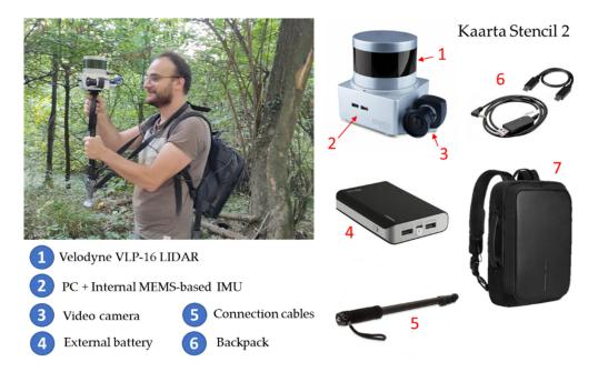
**Figure 7.** Kaarta Stencil 2–16 wearable mobile mapping system used: main components and a photo taken during the data acquisition.
