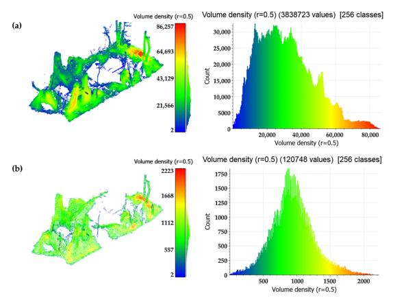
Figure 16. Point cloud density of TLS data and relative histogram (a) with respect to L1 data (b).
