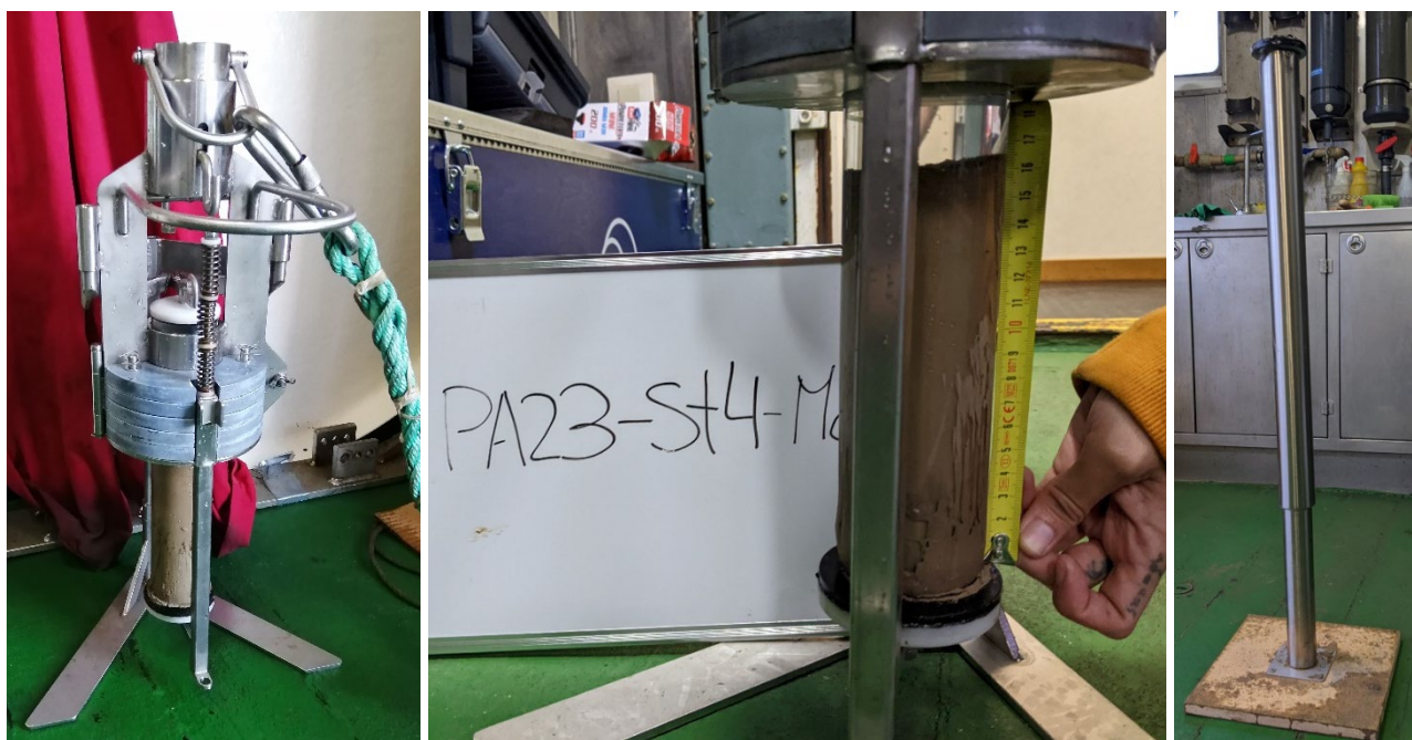
Fig. 31. Sediment sampling with monocrorer. Monocrorer after retrieval (left), monocrorer event recording (middle), and purpose-built extruder for sediment core sampling (right).
