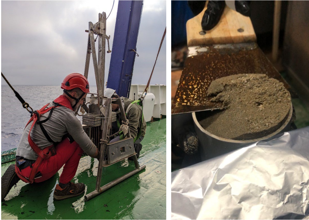
Fig. 32. Sediment sampling with boxcorer. Boxcorer preparation (left) and sub-sampling of pvc tube from boxcorer (right).
