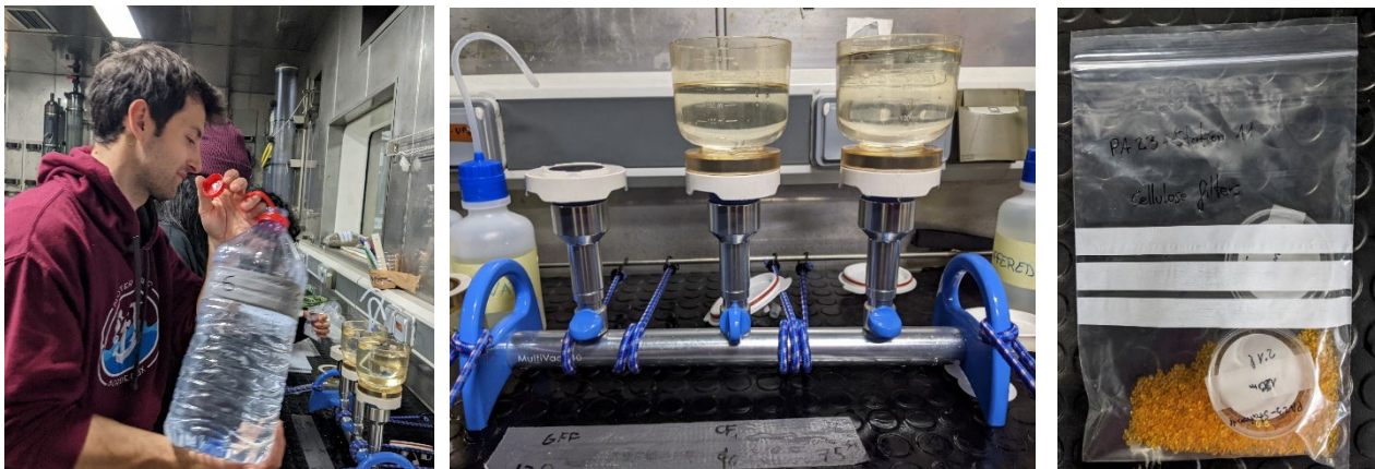
Fig. 29. Sea water filtration for ecological studies. Thibault M. Béjard from the scientific party filtering seawater for ecological studies (left), filtration ramp (middle), and cellulose filters in petri dishes with silica gel (right).
