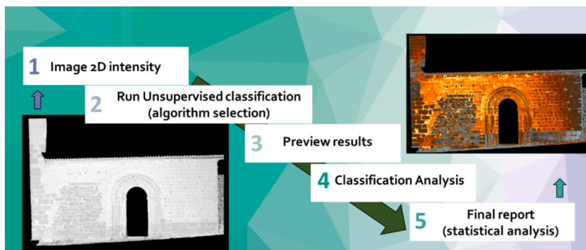
Fig. 7. Schema of the methodology presented once the image intensity is obtained.
