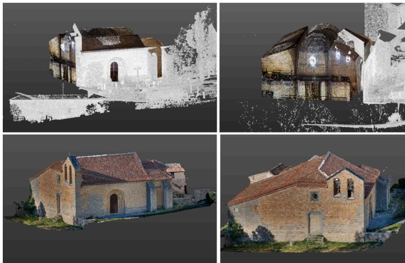
Fig. 4. Top, TLS point cloud. Bottom, point cloud obtained by photogrammetric methods.
