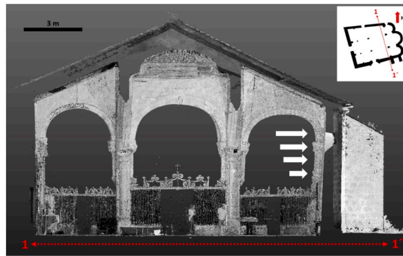
Fig. 12. North-south cross section of the church.
