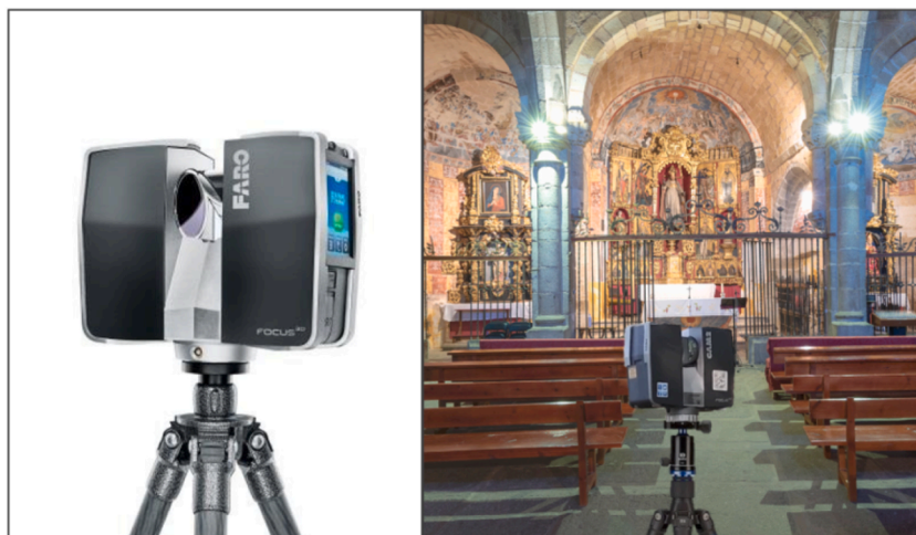
Fig. 2. Detailed view of the Faro Focus 3D 120 Terrestrial Laser Scanner used in this research (left) and during the data collection in the hermitage under study (right).
