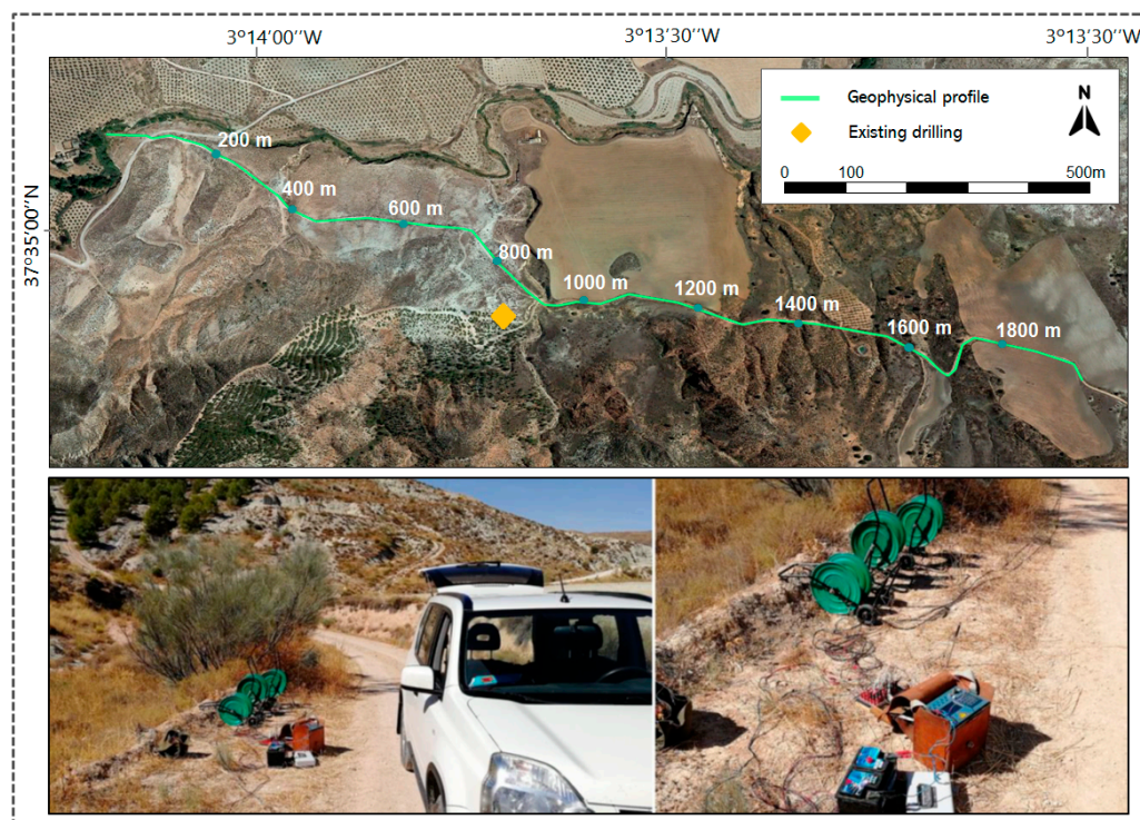
Figure 3. Arrangement of the ERT profile in the area under study (at the top ) execution of works in the field (at the bottom ).
