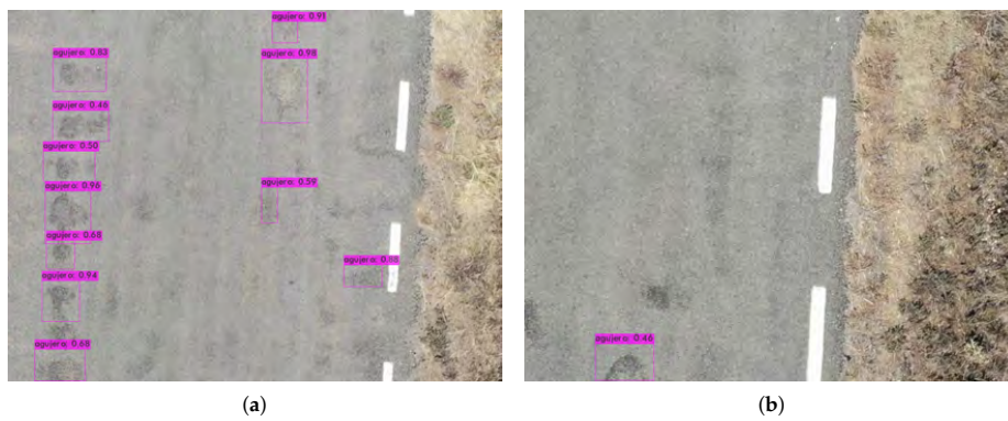
Figure 10. Detection results in a large number of potholes. (a) Multiple detection. (b) Single pothole.
