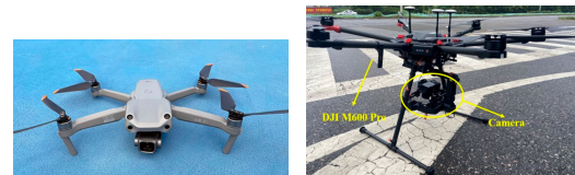
(a) Air 2S is DJI used to adquiry (b) The drone and camera set-up used to capture China_Drone data included in RDD2022.
