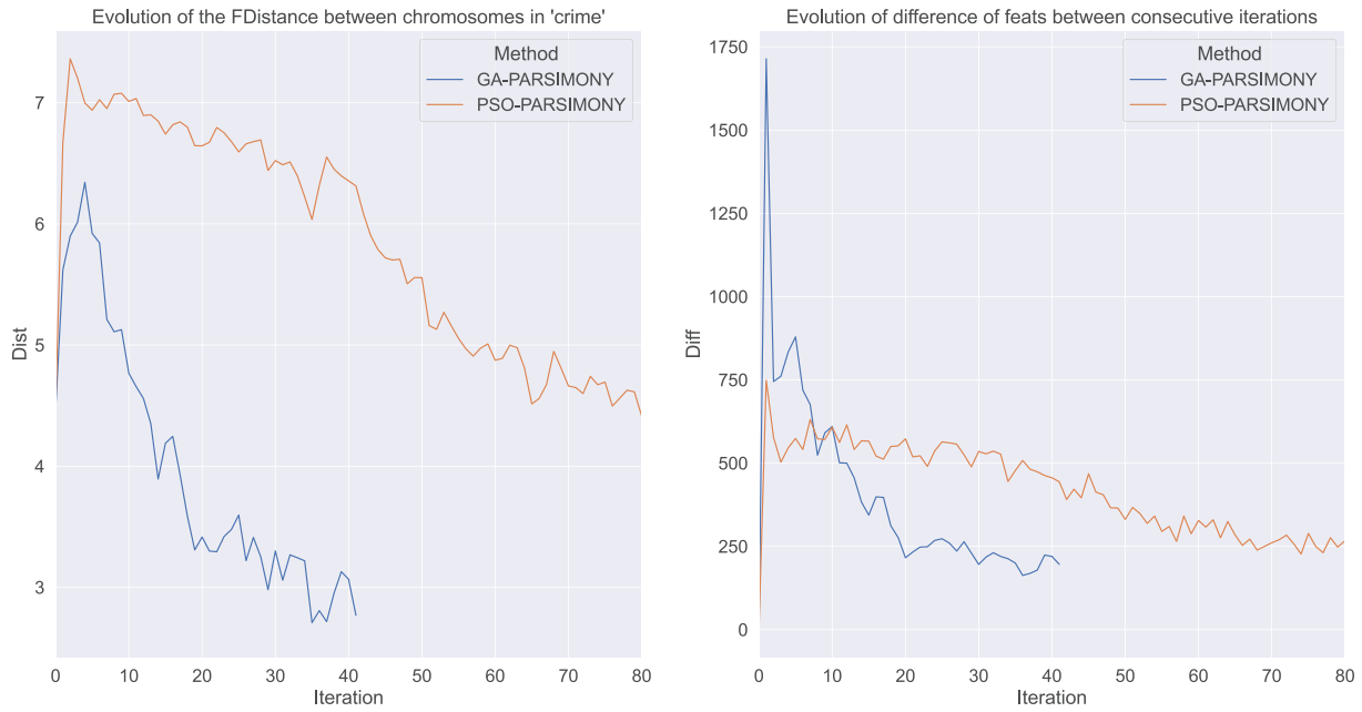
Fig. 1. Evolution of diversity (left) and number of features that change state (selected/unselected) between consecutive iterations (right) with GA-PARSIMONY and PSO-PARSIMONY and crime dataset.
