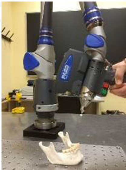
Fig. 4 Arm Scan Platinum model scanner digitalizing the jaw
