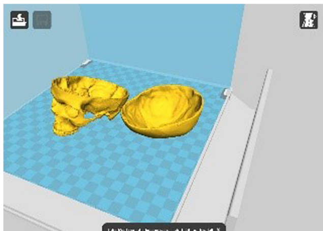
Fig. 7 CURA software interface to create STL formats
