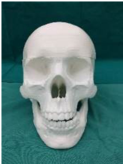
Fig. 9 3D model of the skull printed with polylactic acid (PLA)
