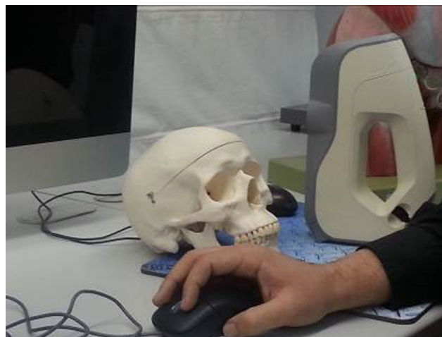
Fig. 2 Hand scanner model Artec Eva used for the digitalization of bone pieces
