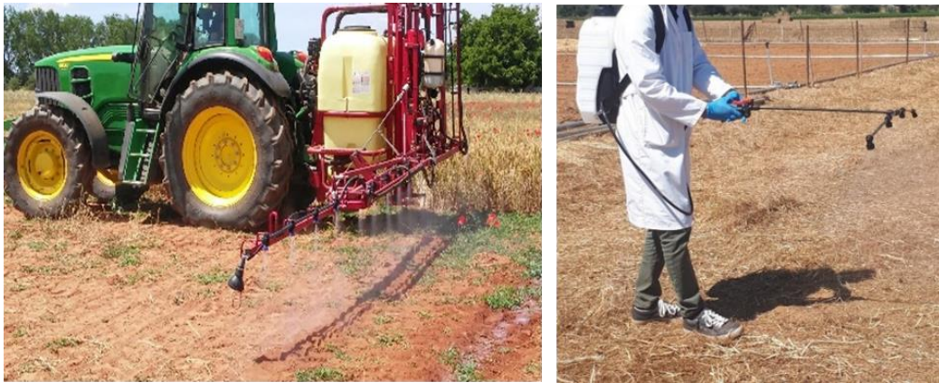
Figure 21. Application of herbicides using a tractor (first application) (left) and an automatic sprayer attached to a backpack (second application) (right).
