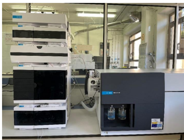
Figure 24. UHPLC-QTOF-MS for herbicide analysis.
