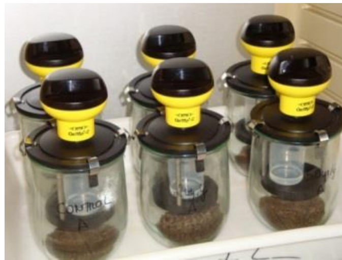
Figure 30. OxiTop measurement system for the determination of the soil respiration.
