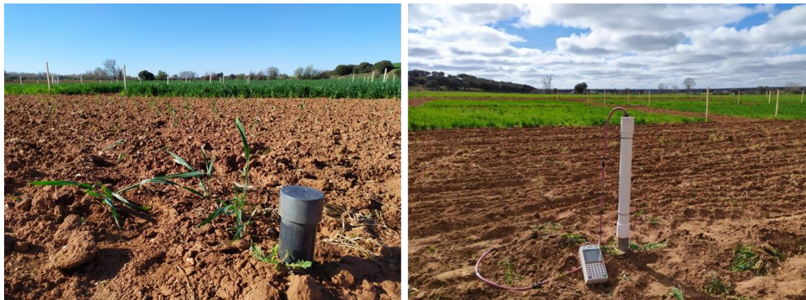
Figure 20. PVC tube installed in the soil profile (left) and Troxler Sentry 200-AP electric probe (right) for measuring the volumetric soil water content.
