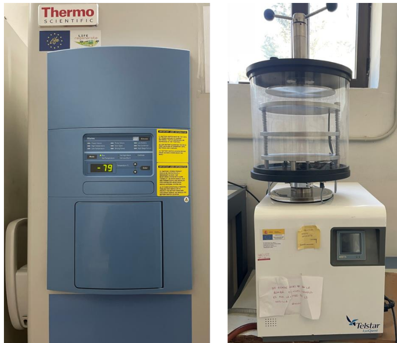
Figure 31. Freezing of soil samples at -79^{\circ}\text{C} (left) and soil sample lyophilization (right).
