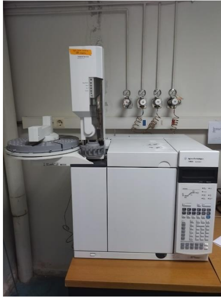
Figure 32. Gas chromatograph coupled to a flame ionization detector (GC-FID) for the quantification of phospholipids (PLFAs).
