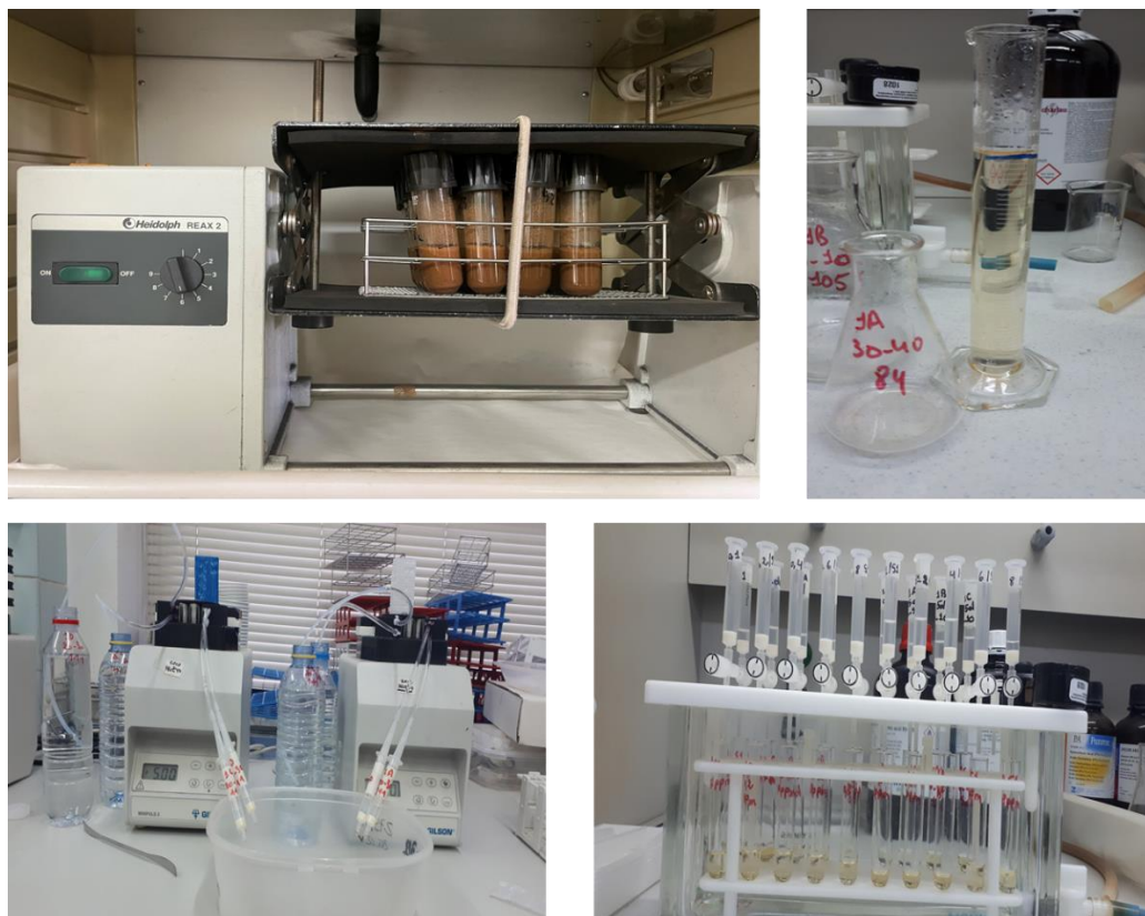
Figure 26. Dissipation and mobility experiment (from left to right, and from up to down): Intermittent shaking of soil samples for 24 h, filtered supernatant, herbicides concentration by solid-phase extraction, and elution of herbicides.
