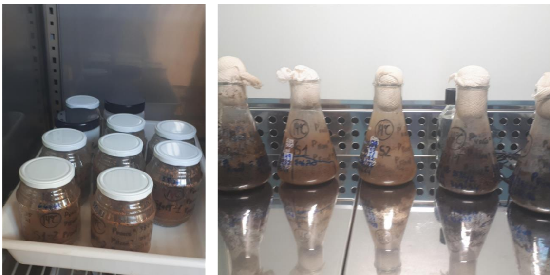
Figure 25. Degradation experiment at the laboratory: Incubation of soil samples at 14°C or 24°C (left), and sterile soil samples in the laminar flow cabinet (right).
