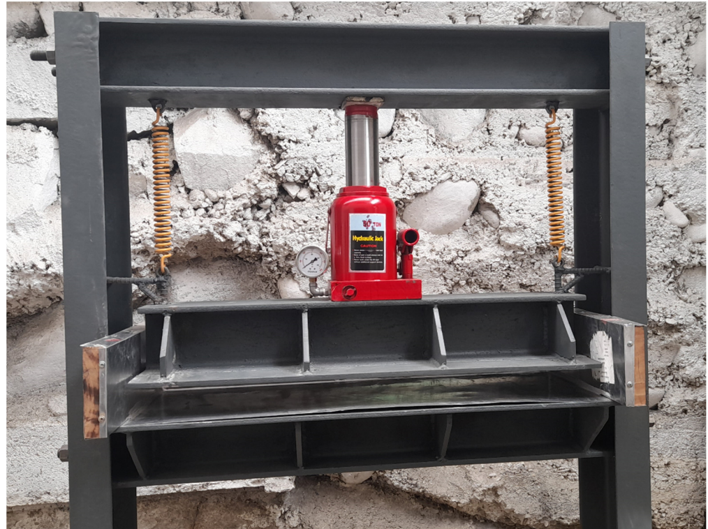
Figure 3. Hydraulic press manufactured for pressing compressed earth blocks.
