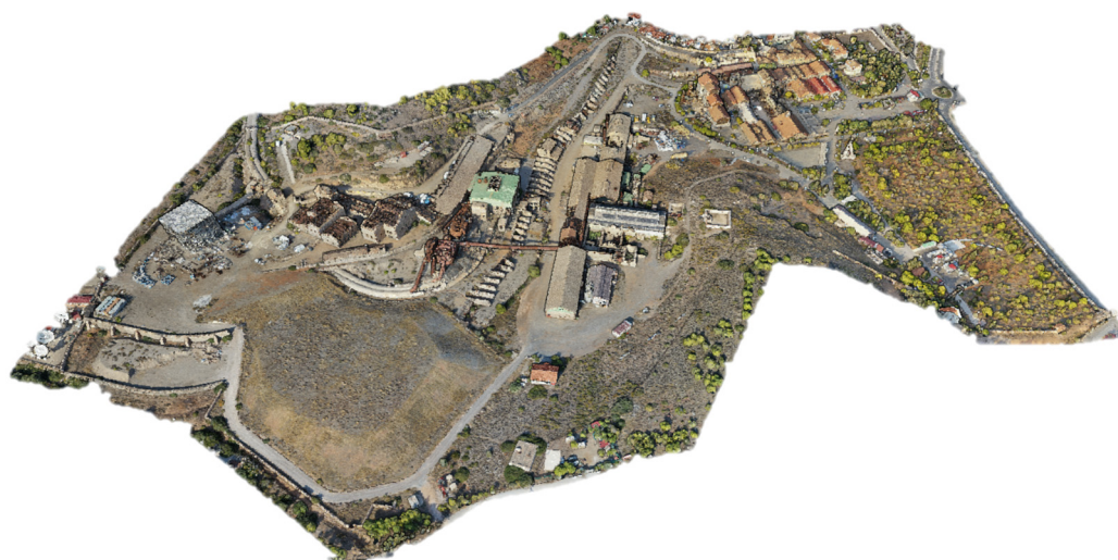
Figure 9. Three-dimensional point cloud generated with the mentioned photogrammetric techniques.
