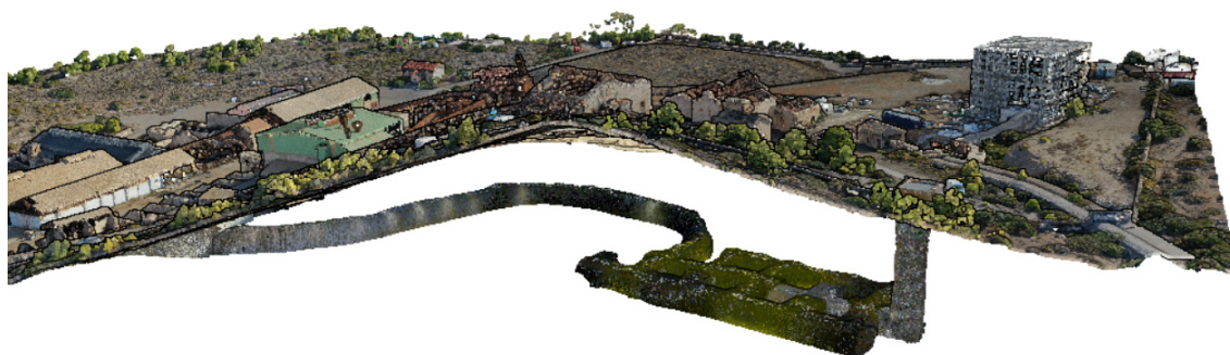
Figure 11. Merged 3D point cloud integrating surface data from aerial photogrammetry and subsurface data from the WMMS.
