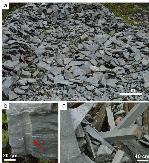
Fig. 2. (a) processing waste (tailings fan) of abandoned serpentinite quarry, Conflenti (Italy), (b) drilling details of serpentinite rock (indicated by the red arrow) and (c) serpentinite rocks cut for construction uses.
