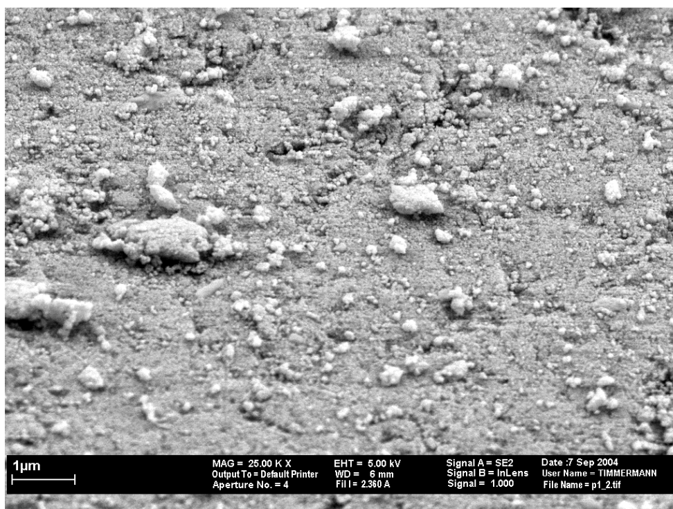
Figure 11. Capillary spraying. P_F = 9.2 MPa; T_F = 314 K; C_{BSA} = 100 mg/cm 3 ; T_{nozzle} = 314 K; P_{nozzle} = 10.4 MPa; q = 70 μl/min.
