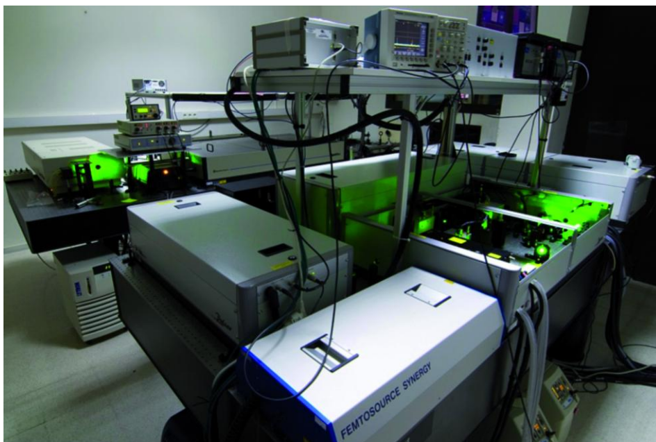
Fig. A.2. Picture of the two laser systems used in the laboratory of ultrafast and ultra-intense lasers of the Universidad de Salamanca. In the front of the photo is the system of Amplitude ( \sim 30 fs), whereas in the rear is the Spectra Physics system ( \sim 120 fs).
