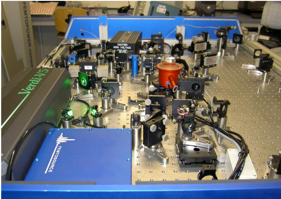
Fig. A.3. Inside view of the amplifier of the laser system (Femtolasers) of the Universitat Jaume I (Castellón).
