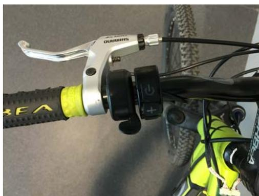
Fig 8. Human-machine interaction device proposed.
