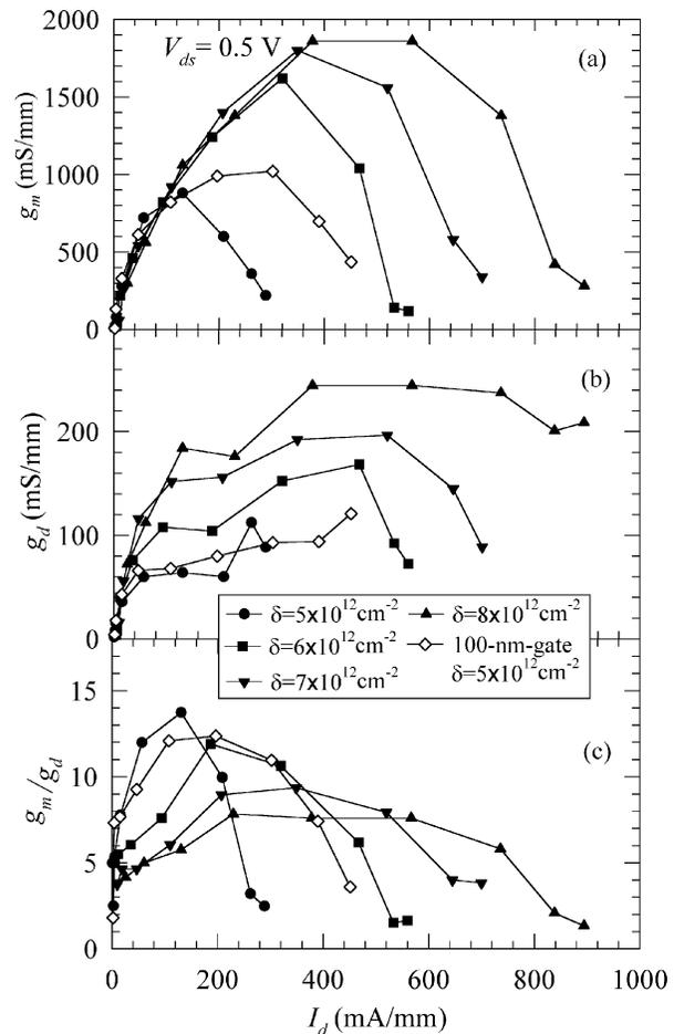
Fig. 6. (a) Transconductance  $g_m$ , (b) drain conductance  $g_d$ , and (c) intrinsic voltage gain  $g_m/g_d$  as a function of the drain current for the 100-nm-gate HEMT and the 50-nm-gate HEMTs with different values of the  $\delta$ -doping. The intrinsic drain voltage is  $0.5 \text{ V}$ .
