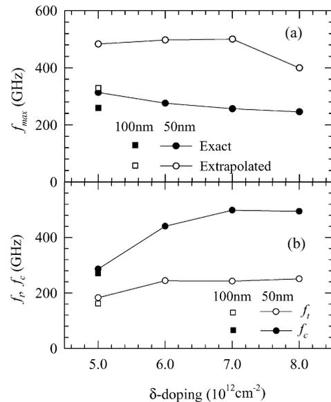
Fig. 10. Maximum values of (a)  $f_{\text{max}}$  and (b)  $f_t$  and  $f_c$  as a function of the  $\delta$ -doping for the 100-nm and 50-nm HEMTs for  $V_{\text{ds}} = 0.5 \text{ V}$  and the  $V_{\text{gs}}$  giving the maximum  $f_{\text{max}}$  (or  $f_t$ ). The width of the devices is  $W = 100 \mu\text{m}$ .
