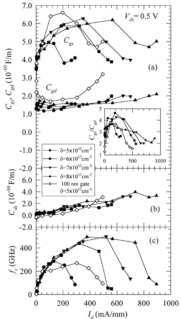
Fig. 8. (a) Gate-source  $C_{gs}$ , gate-drain  $C_{gd}$ , and (b) drain-source  $C_{ds}$ , capacitances and (c) intrinsic cutoff frequency  $f_c$  of the devices as a function of  $I_d$  for  $V_{ds} = 0.5$  V. The inset shows the  $C_{gs}/C_{gd}$  factor.
