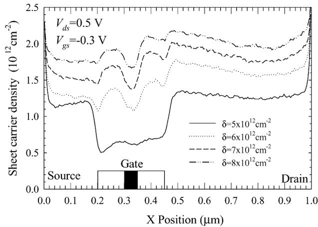
Fig. 7. Sheet-carrier density in the channel of the 50-nm-gate HEMT as a function of the position for different values of the  $\delta$ -doping and  $V_{ds} = 0.5$  V,  $V_{gs} = -0.3$  V. The location of the gate electrode and the recess is also shown.
