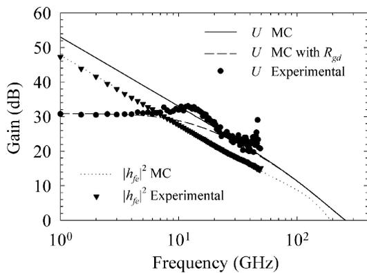
Fig. 3. Values of  $U$  and  $|h_{fe}|^2$  measured in the real 70-nm-gate HEMT and simulated in the 50-nm-gate HEMT with  $\delta = 6 \times 10^{12} \text{ cm}^{-2}$  for the bias point where the maximum  $f_t$  is obtained ( $V_{gs} = 0.1 \text{ V}$ ). Also the value of  $U$  calculated including gate shunt resistance ( $R_{gd} = 60 \text{ K}\Omega$ ) is plotted.
