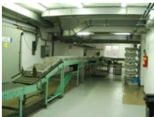
Figure 16. Conveyor of electron beam radiation. Author: Amilcar Antonio.
