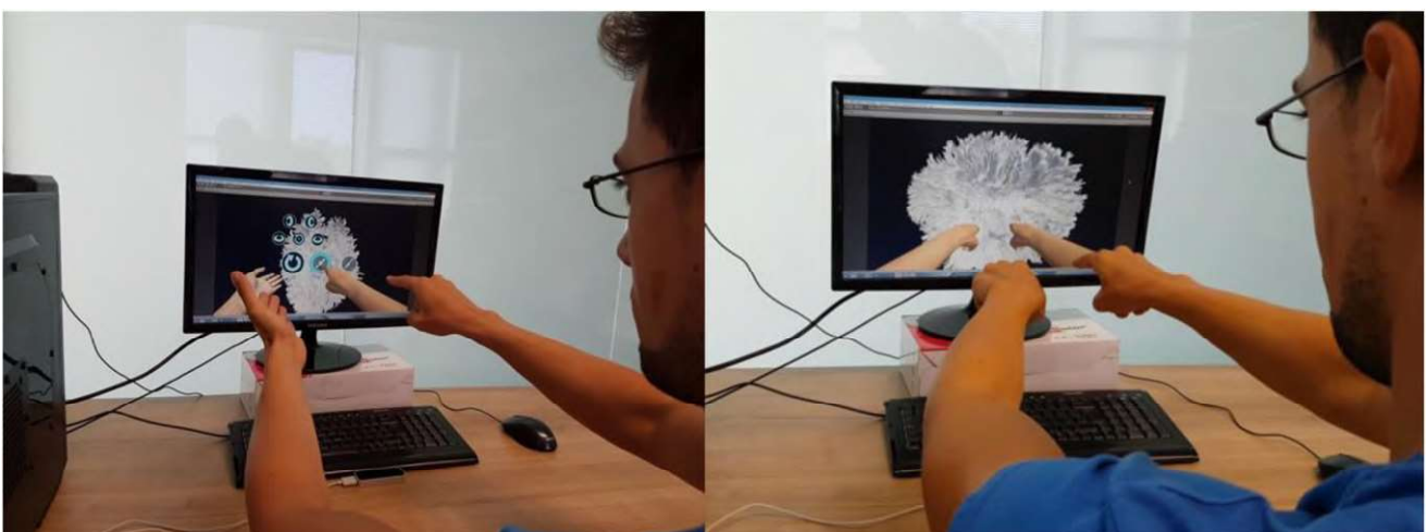
Fig. 4 Manipulating 3D model of brain tracts using hands detection with leap motion
