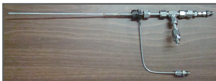
Figura 12. Membrana densa comercial Pd-Ag (50 \mu\text{m} ).
