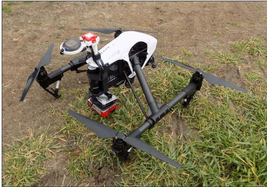
Figure 3.2. DJI Inspire 1 with a hitched Red Edge M camera. GPS receiver and the downwelling light sensor were mounted by using an ad hoc structure.
