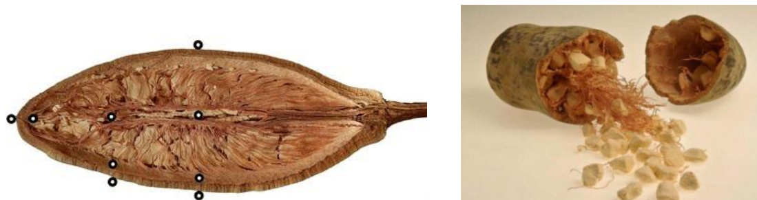
Figure 3. Bisectioned fruits and position of nine thermocouples in A. digitata . Scale bar 50 mm (Kempe et al., 2018).
