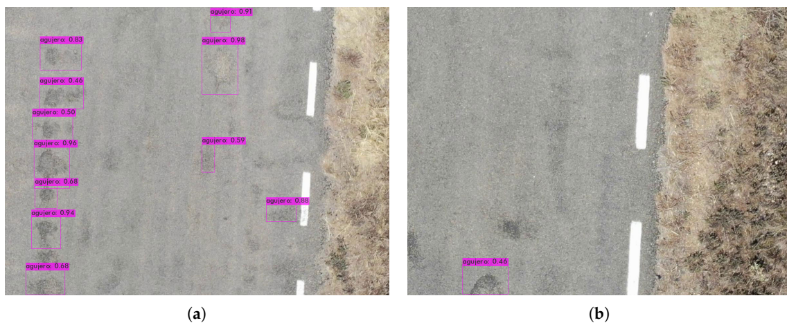
Figure 10. Detection results in a large number of potholes. (a) Multiple detection. (b) Single pothole.
