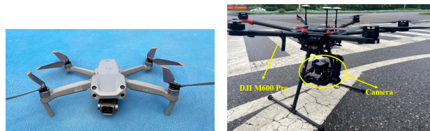
(a) Air 2S is DJI used to adquire images in Spain. (b) The drone and camera set-up used to capture China_Drone data included in RDD2022.
