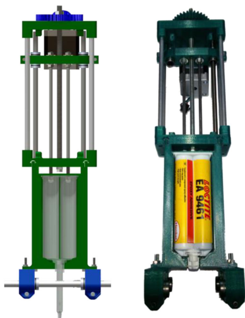
Fig. 3 Image of the adhesive extruder (design and manufacture)
