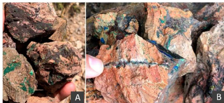
Figure 2. Mineralizations of the Don Jacobo mine; (A,B) Cu carbonates (green and blue colors) and veins of black Co oxides (black colors).
