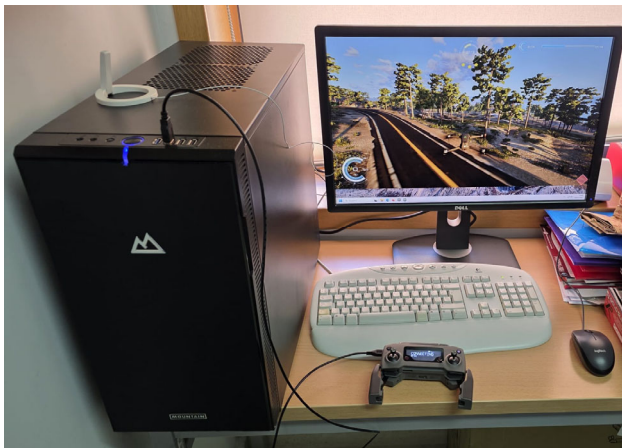
Fig. 2. Simulation workstation used during the immersive UAV training phase, including high-performance computer, professional flight simulation software, and real UAV remote controller. The system enables performance tracking and data collection for learning outcome analysis, supporting the evaluation of maneuver accuracy, mission execution time, and operational decision-making.
