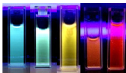
Fig. 13 Fluorescence of the CdS QDs of different sizes (from 2 to 5 nm)
