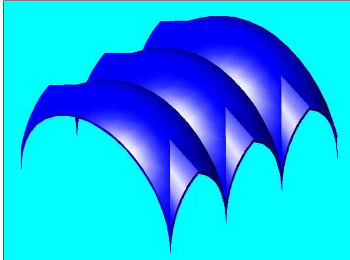
Figure 3: Church of San Ildefonso, in Zamora. Modelling of the vaults.
