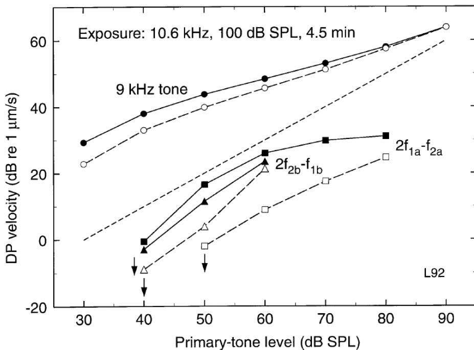
**Figure 1.1.** Example of BM measurement of I/O curves. Filled circles represent an I/O curve for a pure tone at the characteristic frequency (9 kHz) of the recording site. The filled squares and triangles show I/O curves for the  $2f_1-f_2$  and  $2f_2-f_1$  DP components, respectively. The dotted line indicates linear growth. Open symbols represent pure tone and DP I/O curves after noise exposure. Figure taken from Robles *et al.* (1997).
