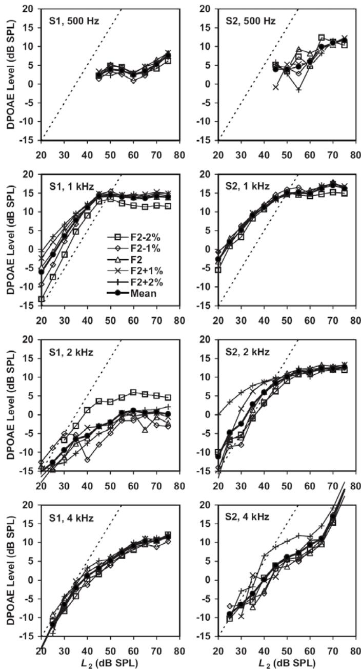
**Figure 2.3.** Example DPOAE I/O curves for subjects S1 (left panels) and S2 (right panels), for frequencies from 0.5 (top) to 4 kHz (bottom) in octave steps. Each final I/O curve (closed circles, thick line) was obtained as the average of five I/O curves for frequencies of  $0.98f_2$ ,  $0.99f_2$ ,  $f_2$ ,  $1.01f_2$ , and  $1.02f_2$ , illustrated with different symbols according to the inset. The dashed line illustrates a linear response for comparison.
