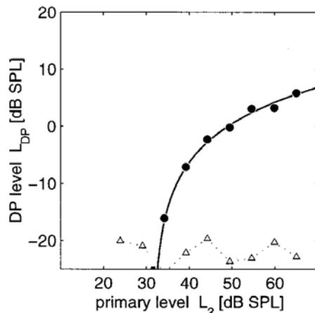
**Figure 1.2.** A typical DPOAE I/O curve for a normal hearing subject (filled circles and solid line). Open triangles represent the measurement noise floor. Figure taken from Boege and Janssen (2002).
