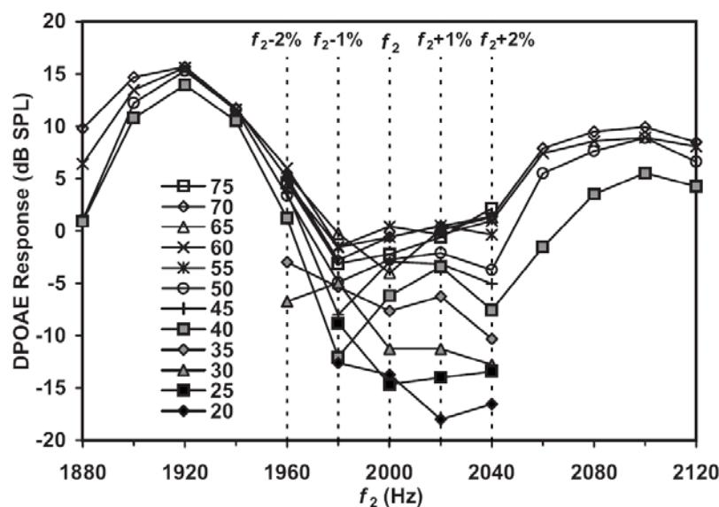
**Figure 2.2.** An example of the influence of the DPOAE fine structure at 2 kHz. An example data set recorded to estimate every I/O curve is also illustrated. The DPOAE magnitude is shown for 12  $f_2$  frequencies around the frequency of interest (2 kHz) and for different  $L_2$  levels (in dB SPL) as indicated in the inset.
