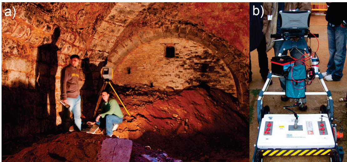
Figure 2. (a) Terrestrial laser scanner used for the recording of the external geometry, Trimble GX; (b) ground penetrating radar equipment, RIS MF HI-MOD 200–600 MHz.
