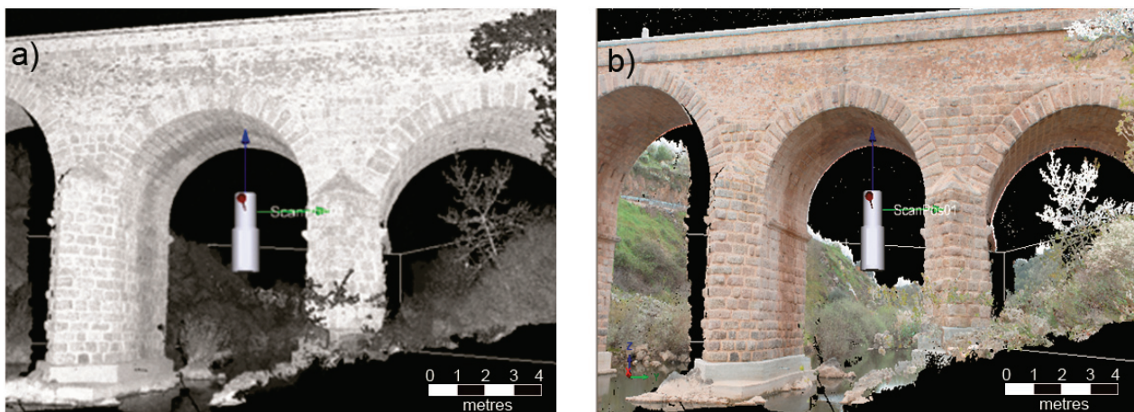
Figure 4. Visualization of a 3D point cloud as a function of (a) the intensity of the reflected laser beam or (b) the photorealistic texture of the object.
