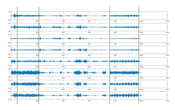
Figure 2: 8 channels of EMG signals corresponding to two different gym exercises (separated between vertical lines) and null-data between the exercises.
