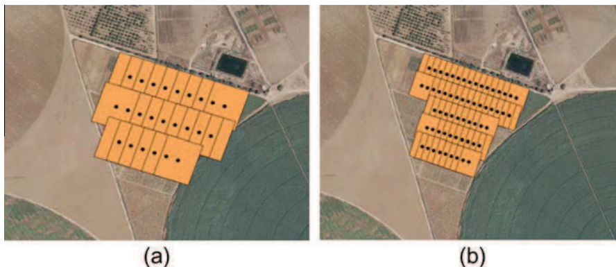
Fig. 2. Flight planning of 0.15 m GSD (at 245 m height) (a) and 0.08 m GSD (at 145 m height) (b).
