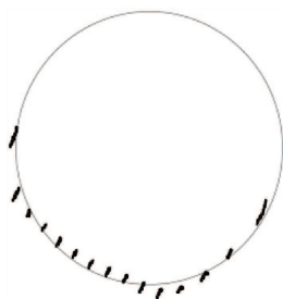
Figure 4: An estimation of the Diameter at Breast Height (DBH) is obtained by fitting a circle to projected trunk points of an appropriate portion of the trunk.
