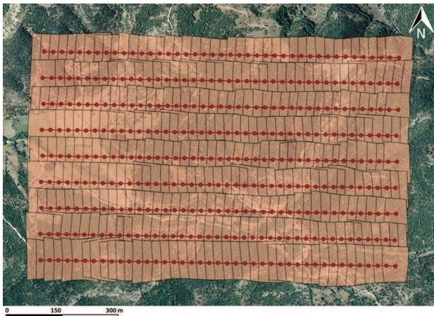
Fig. 6 Flight planning, 0.08 m GSD: rectangles represent the footprint of each image, and circles are the camera positions along the flight strips (EPSG code 25830)
