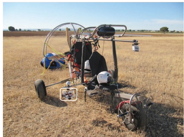
Fig. 1 Aerial photogrammetric platform (PPG trike) with the gimbal shown (white rectangle)
