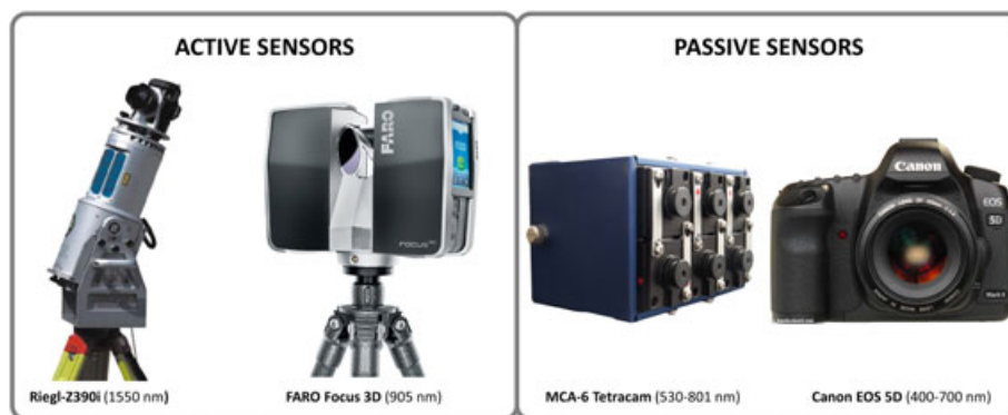
Figure 2. Sensors used for data collection. From left to right as active sensors: RIEGL-Z390i and FARO Focus 3D. As passive sensors: MCA6 Tetracam and Canon EOS 5D.
