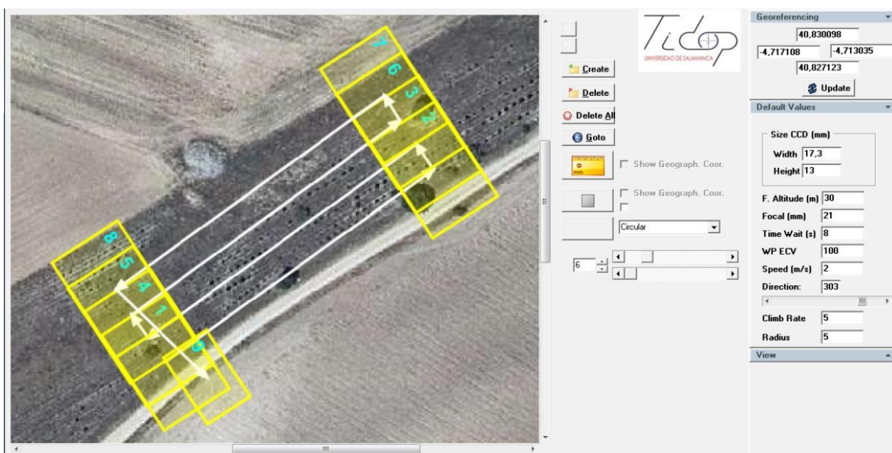
Figure 4. Photogrammetric flight planning using an orthoimage of the study area.
