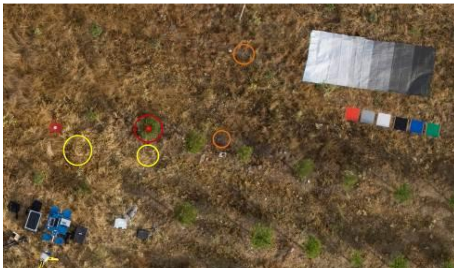
Figure 8. Aerial image of the control and check surfaces.
