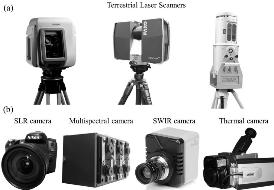
Figure 6. Examples of sensors used in the inspection of constructions: (a) active sensors, (b) passive sensors.
