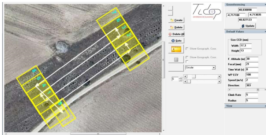
Figure 4. Photogrammetric flight planning using an orthoimage of the study area.
